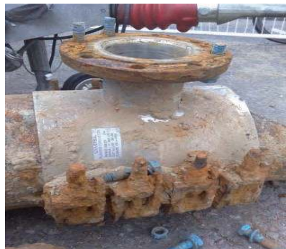
Ductile lugged UPT removed from the ground
