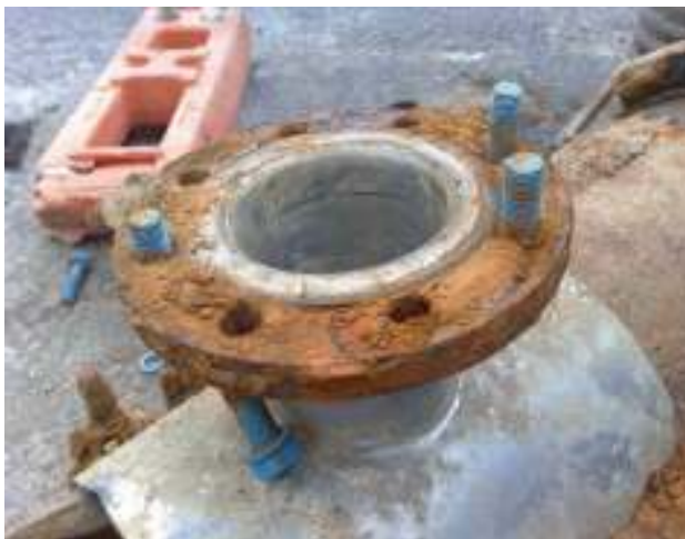
Ductile lugged UPT removed from the ground
