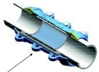
■ The Cascade PE Clamp/Coupling can be used to join pipes with a large gap due to the length of the fitting, particularly where Electro-fusion couplings have been cut out (As in above picture).
